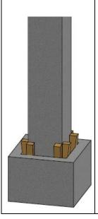
After the position was established, the wooden wedges are used to temporarily fix the columns. The wooden wedges will also help to make more positioning adjustments before in order to fill with concrete and permanent fixing.
