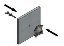
The column connector is fixed to formwork using a threaded bar and two wing nuts.
