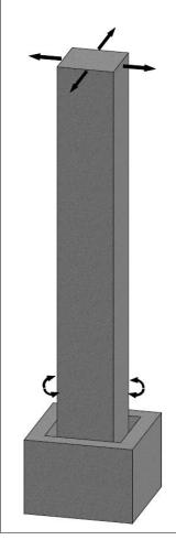
The connectors permit the column to pivot and maintain a fixed contact point.
